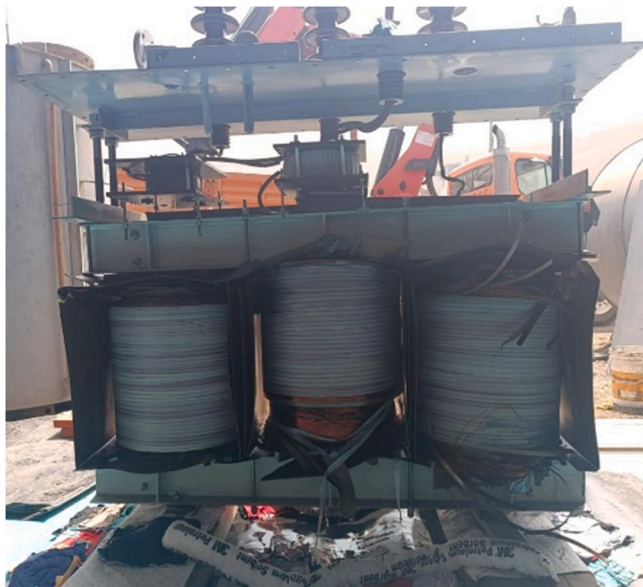
Fig. 10. Internal laboratory inspection with the fault in the phase B in the zig-zag transformer, for the case study.
