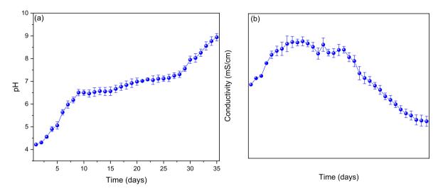
Fig. 3. Values of (a) pH and (b) electrical conductivity of microbial fuel cells during monitoring.
